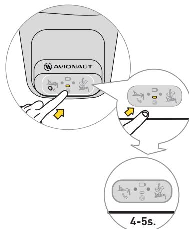
To mute the sound, press the display button for 4-5 seconds. The display will still show the correct/incorrect seatbelt and base attachment, but the sound will be muted.
