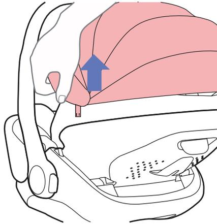
You can remove the hood by pulling it from the sides. To reinstall it, insert the two terminals into the housing behind the eyelets in the upholstery.
