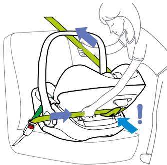
Pass the shoulder portion of the belt over the baby's head and insert it into the guide slot (9) in the backrest. Pull the belt tight and let your car's retractor take up the excess slack. Check that the belts are not twisted or loose.
