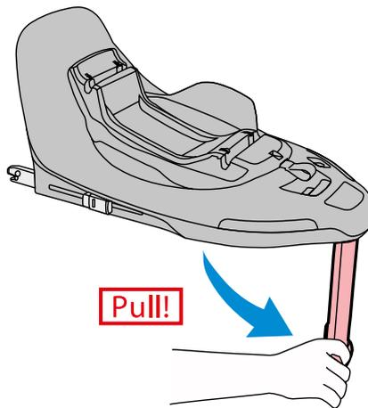
Unfold the support leg (19) from its compartment.
