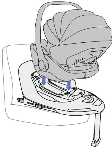
Store the baby carrier on the base trying to route both axles of the baby carrier onto the 4 anchors of the base.
