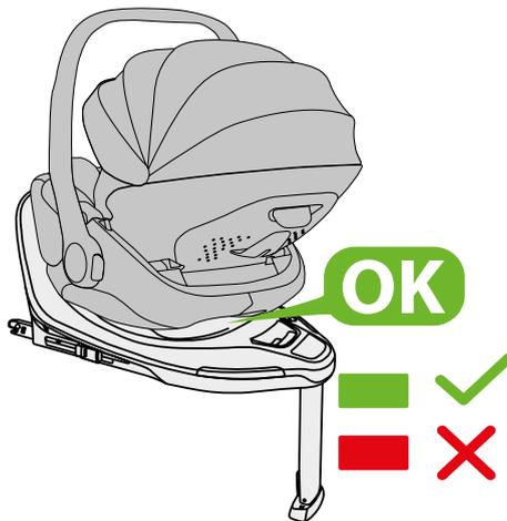
If it has been properly anchored, a green signal will appear on the anchorage indicator (17). To make sure, pull the carrier up.
